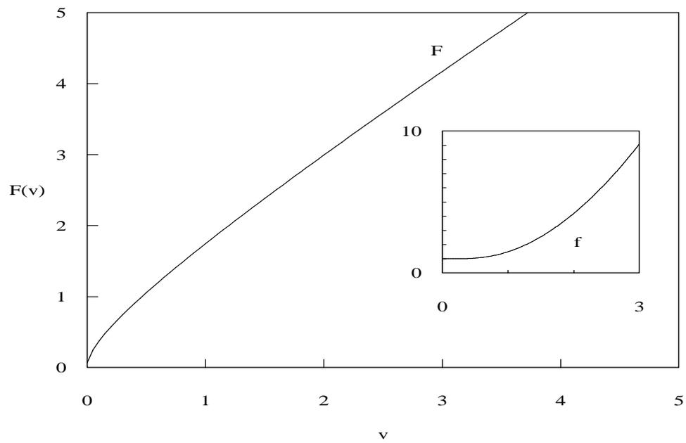
**Figure (1)** The potential  $f(x) = x^2 + 1/(1 + x^2)$  is shown in the inset graph, along with the corresponding ground-state energy function  $E = F(v)$ . The aim of geometric spectral inversion is to reconstruct  $f$  from  $F$ .
